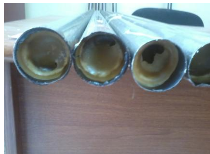
Fig. 2. A photo of the paraffin wax inside the pipes
